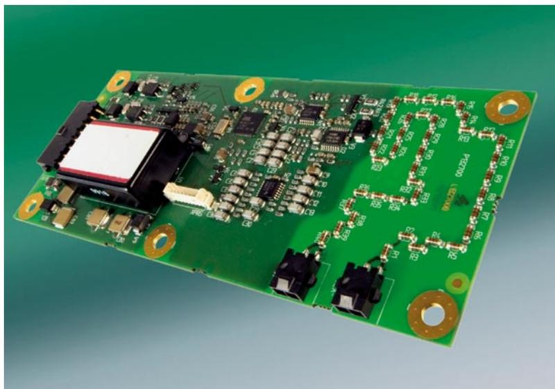
**Figure 3:** Circuit board version of an insulation monitoring device, weighing 50 g, according to DIN EN 61557-8 (VDE 0413-8), with a temperature range of -46 °C to 105 °C (125 °C for 3 h)
