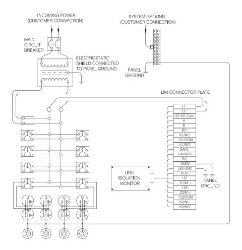
NOTE: Typical schematic. Quantity of receptacles and ground jacks may vary by application.
