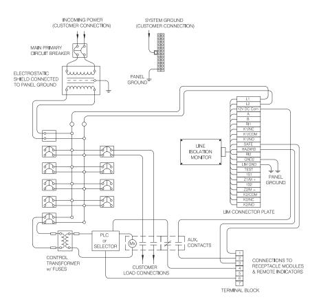
NOTE: Typical schematic. Quantity of circuits controlled by PLC may vary by application. Connections may vary when controlled by selector.
