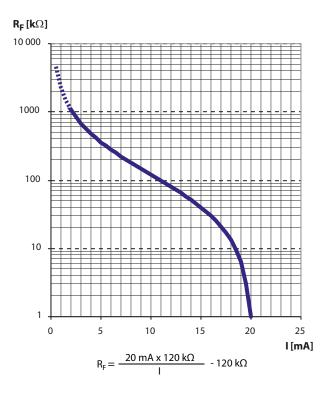
$R_F$  =Insulation fault in  $k\Omega$ I =Current output in mA
