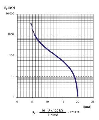
$R_F$  =Insulation fault in  $k\Omega$ I =Current output in mA
