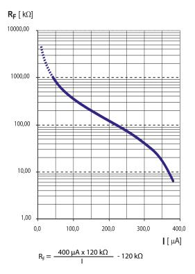
$R_F$  =Insulation fault in  $k\Omega$ I =Current output in mA
