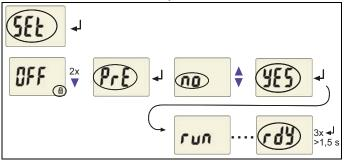
If loop resistances of approx.  $\geq$  1 k $\Omega$  exist, the preset function will be ineffective. The message "AL not SEt" appears on the display.
