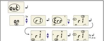
Alarm relay 1: Deactivating the category measuring current disconnection
