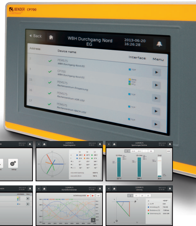
Representation of device data on the touch screen (COMTRAXX® CP700)
