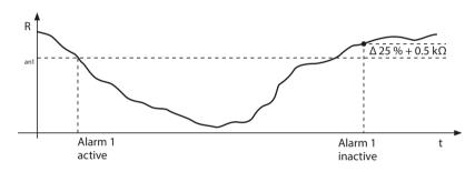
An alarm will become inactive as soon as +25 % +0.5 k $\Omega$  of the set operating value is exceeded.
