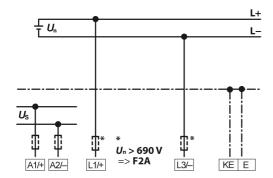
In systems with a nominal system voltage of more than 690 V and with overvoltage category III, a fuse for the connection to the system to be monitored must be provided. \* 2 A fuses recommended.
