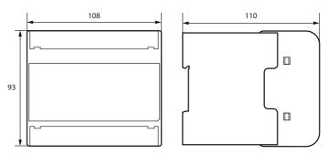
Img.: Enclosure iso685...-device familiy – dimensions in mm
