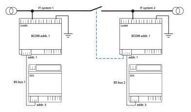
Via the X1 connector, the ISOMETER® can be isolated from the IT system and the measuring functions can be deactivated. Therefore, the function of the digital input in use has to be set to Device inactive.
