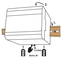
Img. 4-3: DIN rail mounting
