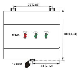
Img. 4-2: Screw mounting; dimensions in mm (in)
