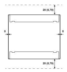
Img. 4-1: Mounting spaces; Dimensions in mm (in)
