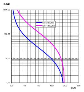
$$R_F = \frac{20 \text{ mA x R}_{Sk}}{I} - R_{Sk}$$
