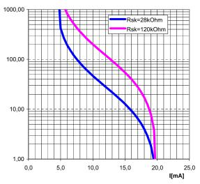
$$R_F = \frac{-16 \text{ mA x R}_{Sk}}{\text{I - 4 mA}} - R_{Sk}$$
