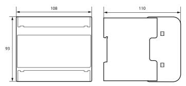
Figure: Enclosure iso685...-device familiy – dimensions in mm
