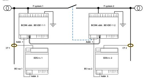
Each ISOMETER® iso685-x-P manages its EDS devices and sends its EDS devices the trigger signals required for insulation fault location via its BS and BB bus. The EDSsync function must be activated so that EDS devices which are connected to other iso685-x-P can also receive trigger signals in coupled systems.
