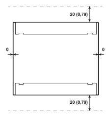
Figure 4-1: Mounting spaces; Dimensions in mm (in)
