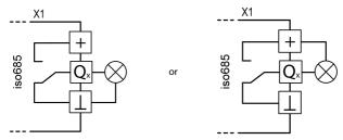
• Passive In passive mode, ≤ 32 V are connected externally (see technical data). The output switches the applied potential to ground.
