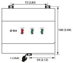
Figure 4-2: Screw mounting; dimensions in mm (in)
