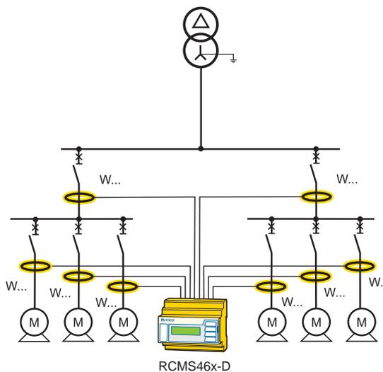
*BENDER's ground fault location systems find faults without shutting down*
