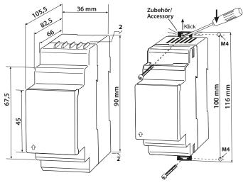
The front plate cover is easy to open at the lower part identified by an arrow.
