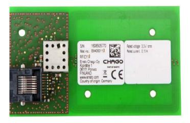
For use in combination with charge controllers used in electric vehicle charging stations, wall boxes and street light charging points
