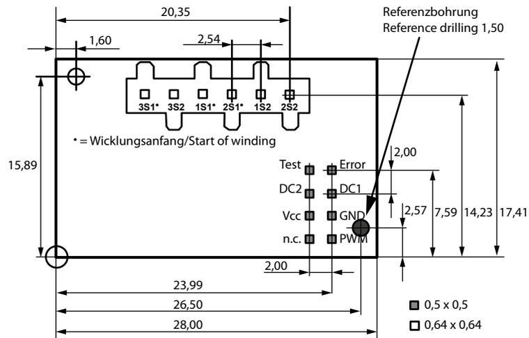
**Connection socket measuring current transformer**
