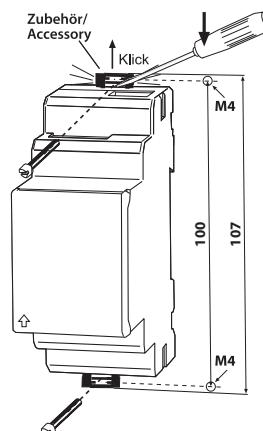
The front plate cover can be opened by raising the lower part marked with an arrow.
