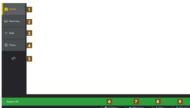
The alarm bar (displayed in green) is visible on every dashboard. This is required by the standards. If a fault occurs, a message window appears and an acoustic signal is output. The *Cleaning Mode* locks the touch screen for 20 seconds to prevent unwanted operation while the screen is being cleaned. The links allow the user to switch between the user interfaces
